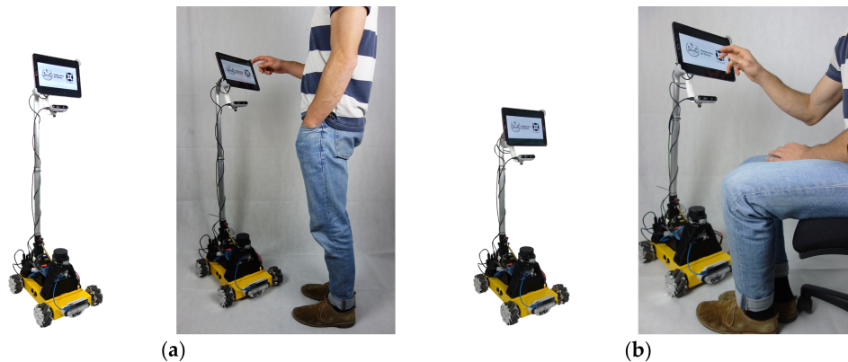
Fig. 6.4 Final prototype of the mobile assistive robot in two different working configurations: (a) Deployed configuration for standing usage, HMI height = 1.1 m, mechanism tilting angle = 0^\circ , (b) Retracted end angled configuration for better-seated usage, HMI height = 0.80 m, mechanism tilting angle = 20^\circ .
