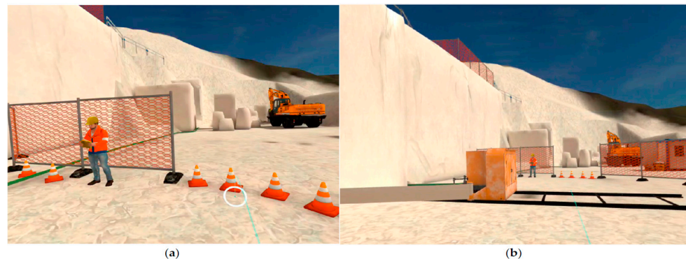
Figure 17. VR training for primary upstream cutting (SO1): safety-distance verification (a) and positioning of diamond wire guards before horizontal cutting (b). Reproduced from [89], © 2025 The Author(s), distributed under the Creative Commons Attribution License (CC BY 4.0).
