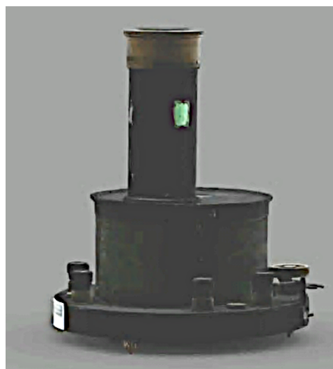
Fig. 6. UVL texture applied to the same 3D model of Fig. 5. Areas of luminescence reveal possible coatings or degradation residues.
