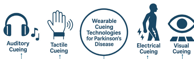
FIGURE 1. Wearable Cueing Technologies for PD from left to right: auditory cueing, which uses rhythmic sounds such as metronomes or verbal cues to regulate gait timing; tactile cueing, providing haptic feedback through vibration to assist movement initiation; electrical cueing, which delivers proprioceptive electrical impulses to trigger or correct motor responses in real-time; and visual cueing, employing visual prompts like floor lines or laser guides to enhance step length and coordination.
