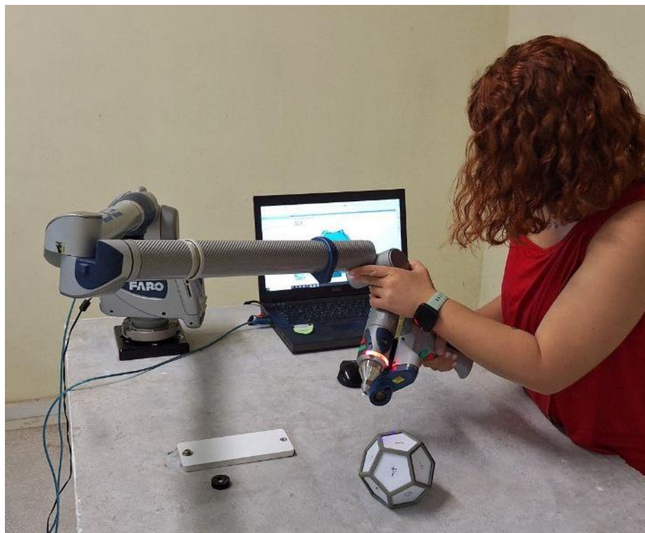
Figure 6.7 FARO Laser ScanArm Edge during the acquisition of the dimensional reference.
