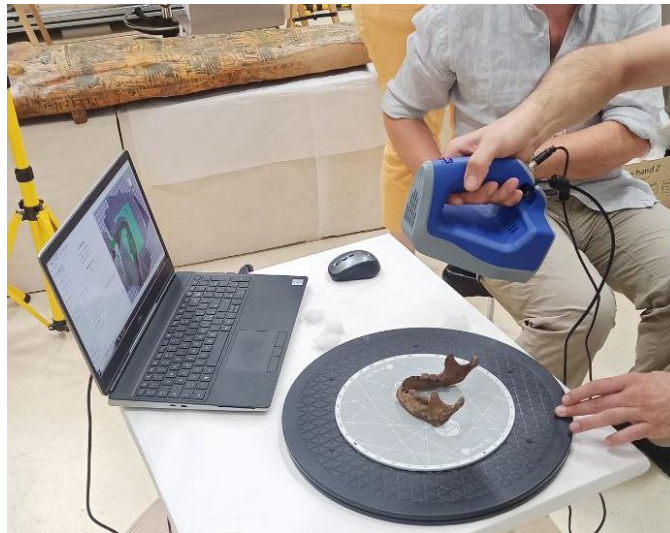
Figure 8.17 Acquisition setup Acquisition setup for the reconstruction of the skull's 3D model by 3D scanning.
