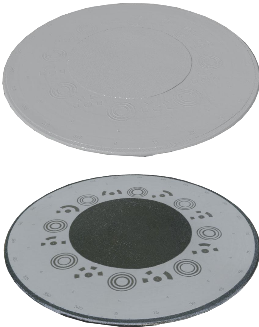
Figure 5.2 3D virtual replica of the platform: above is represented the mesh, and, below, the texture.
