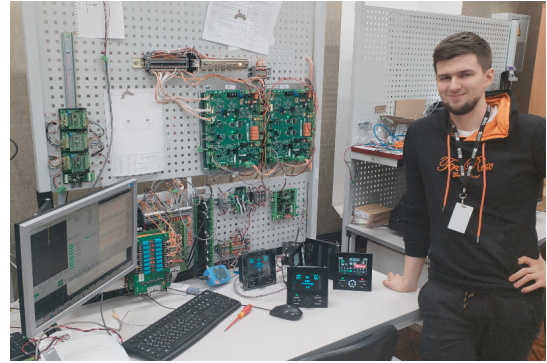
Fig. 5. Testbench (HIL) of roll damping system
