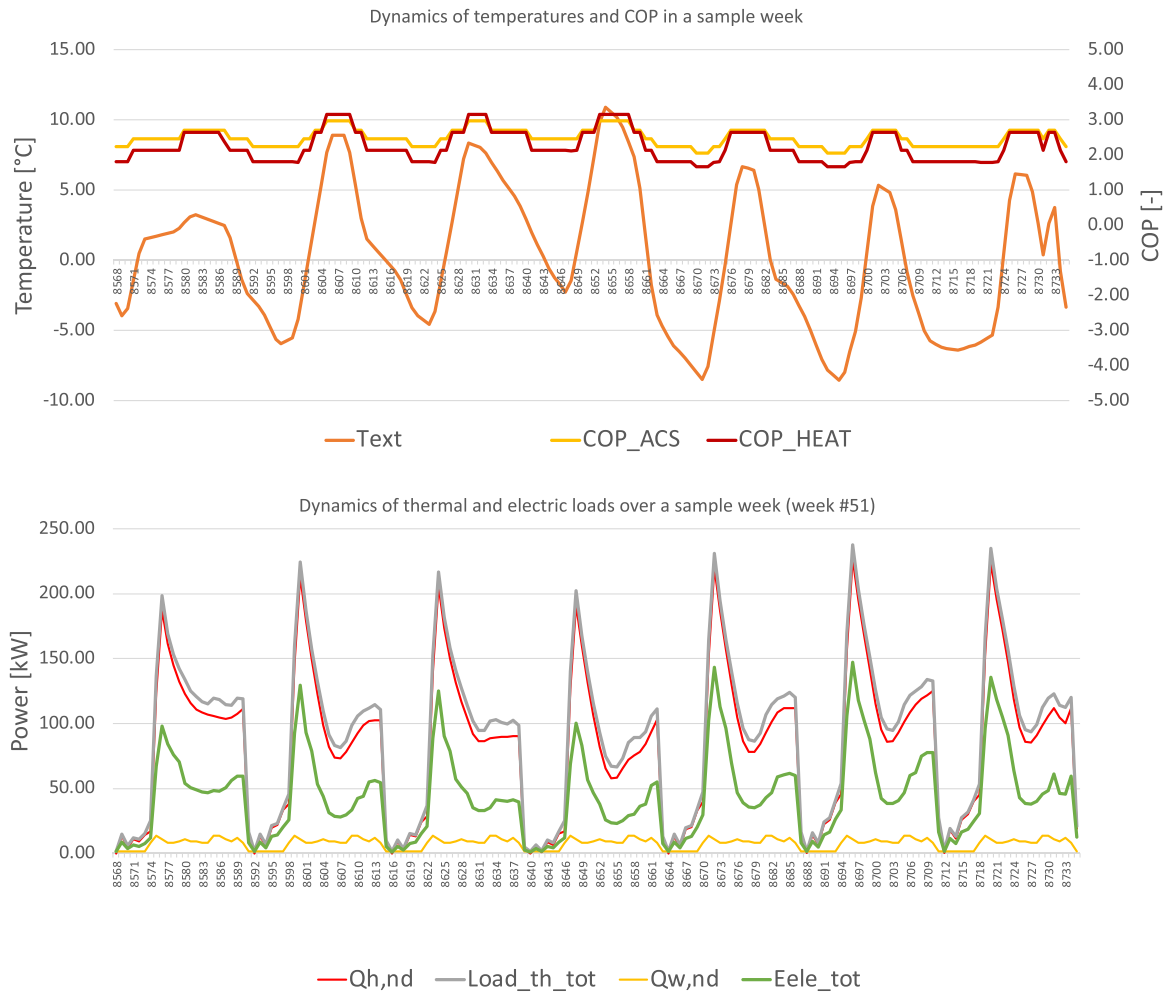
Fig. 11. Dynamic hourly operation of the analysed R-290 heat pump over a sample week (week 51): top - COP values (HP-modules for space heating in relation to external temperatures; bottom - electrical power (yellow) and COP values for heating and DHW (grey and blue, respectively).
