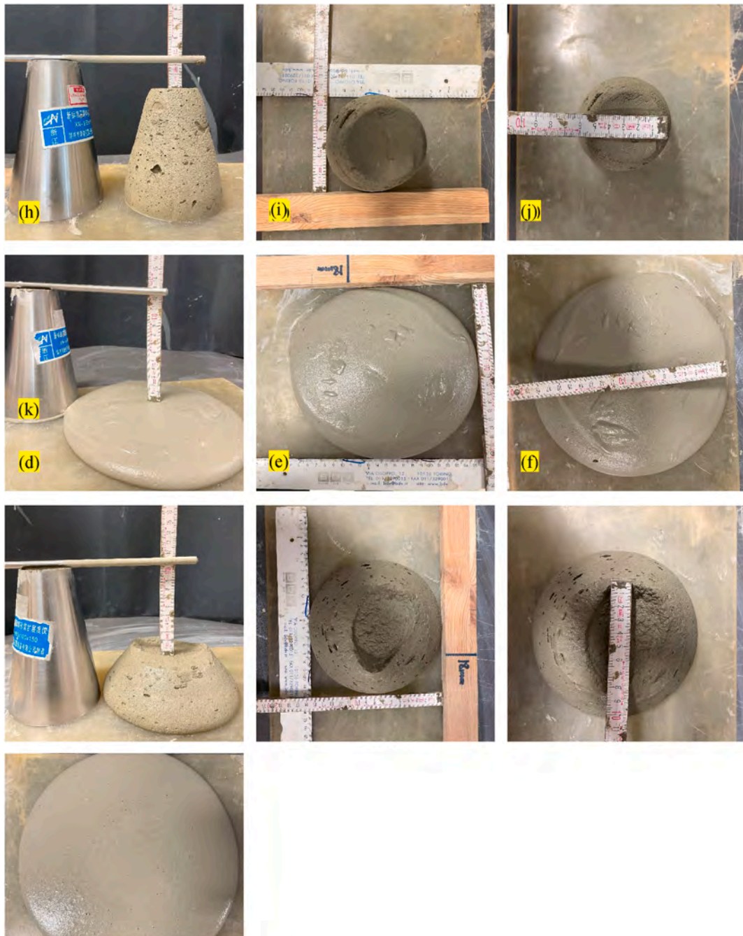
Fig. 7. Slump values of foamed concrete for different maximum fine sand particle size and with or without metakaolin. (âc) S1P3; (d ~ f) S1P3K; (h ~ j) S2P3; (k) S2P3K.
