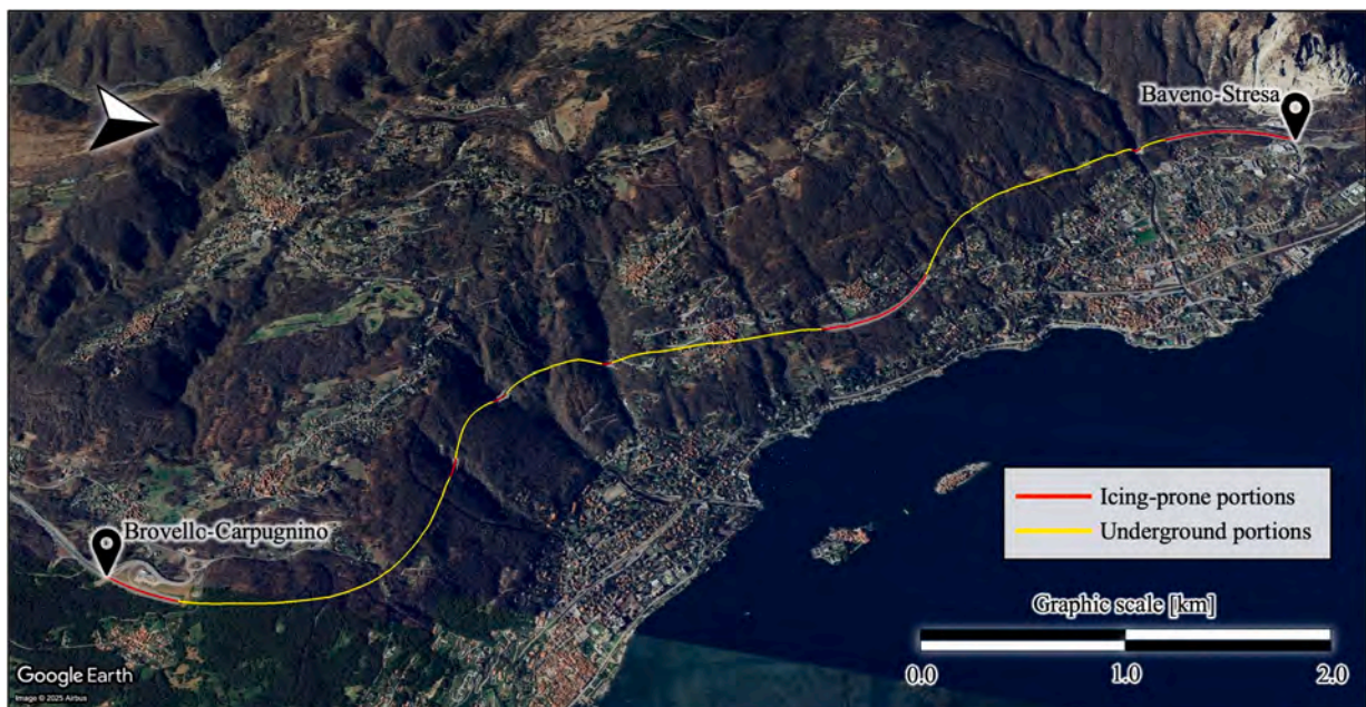
Fig. 13. A26 motorway stretch from Baveno-Stresa to Brovello-Carpugnino and identification of the icing-prone and the underground motorway portions.
