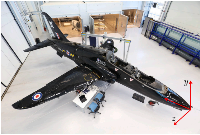
Fig. 8. BAE Systems Hawk T1A aircraft experimental setup at the LVV at the University of Sheffield, showing the reference frame and its origin (adapted from [41]).
