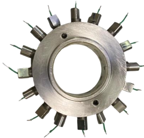
Figure 8.4 Oedometer ring with flat-shaped electrodes.
