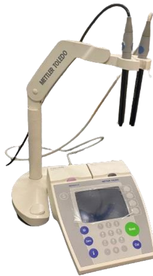
Figure 4.17 Conductivity-meter from Meter Toledo used for electrical conductivity and pH measurements.
