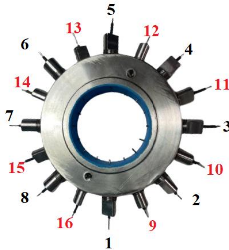
Figure 8.3 Oedometer ring with 3D plastic insulation and electrodes. Black numbers refer to top level electrodes, and red numbers refer to bottom level electrodes.
