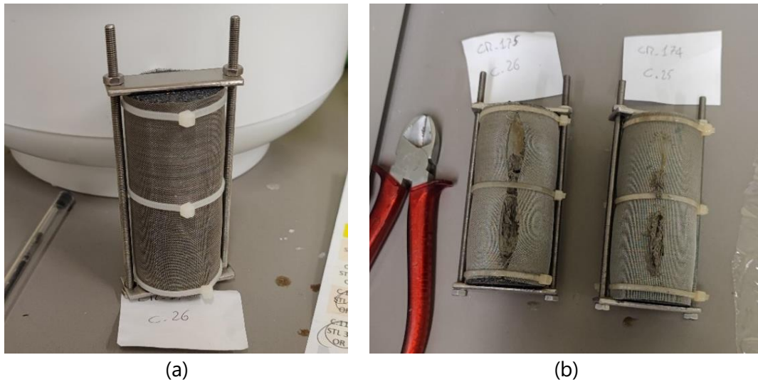
Figure 6.31 Reconstituted samples and cages along with the samples of Clay B material exposed to CO 2 -saturated brine (a) before exposure and (b) after exposure.
