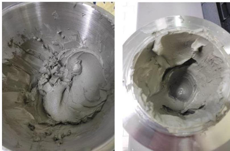
Figure 4.10 Placement of powder paste in the reaction chamber before exposure to \text{scCO}_2 .
