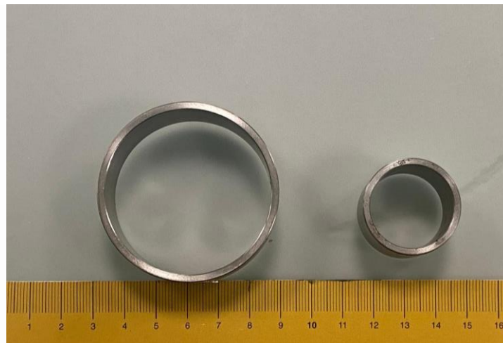
Figure 4.13 Sample rings for the standard oedometer on the left and small diameter oedometer on the right.
