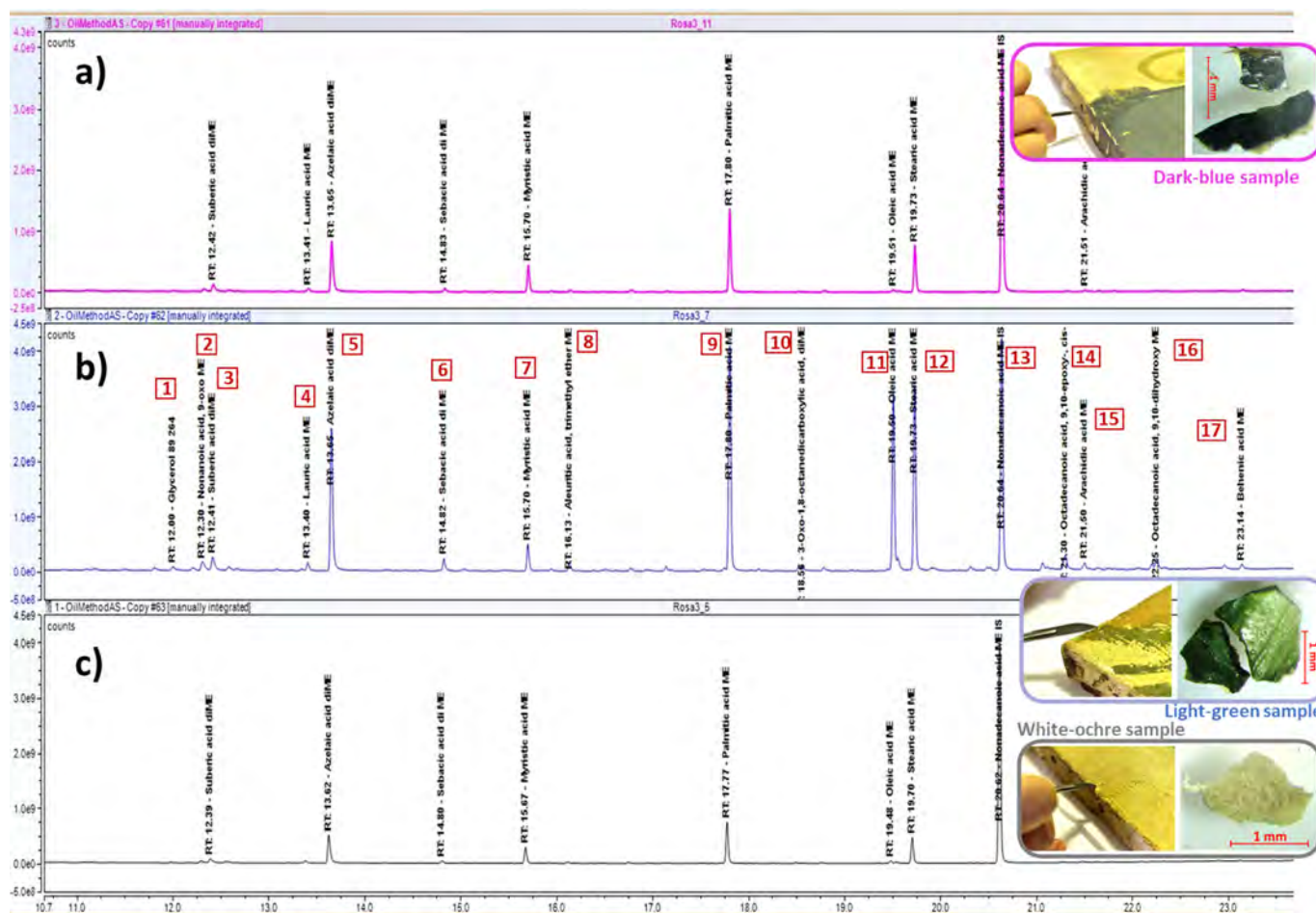
Figure 11. Total Ion Current (TIC) chromatograms after derivatization and analysis through GC-MS of (a) dark blue; (b) light green; and (c) white-ochre fragments. Ascending numbers are associated with the peaks in the chromatogram obtained for the green sample: the same ones are used in Table 1 to help data visualisation. Photographs of the sites of sampling and of the magnified fragments are shown too.
