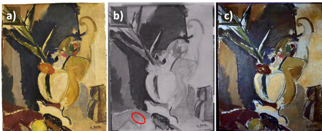
Figure 6. (a) Visible light, (b) IR reflectography (950 nm high-pass filter) with pentimento circled in red, and (c) UV-induced fluorescence images of the entire painting.
