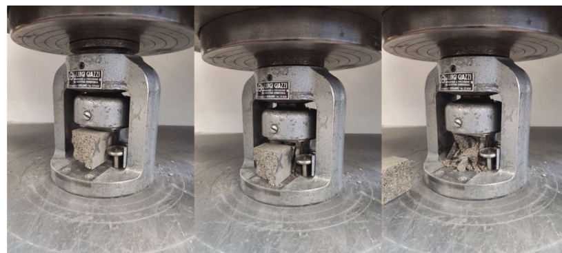
Figure 3. Compressive test of mortar specimens.
