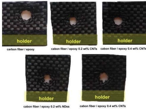
Figure 3: Photographic images of composite specimens after ablation testing.
