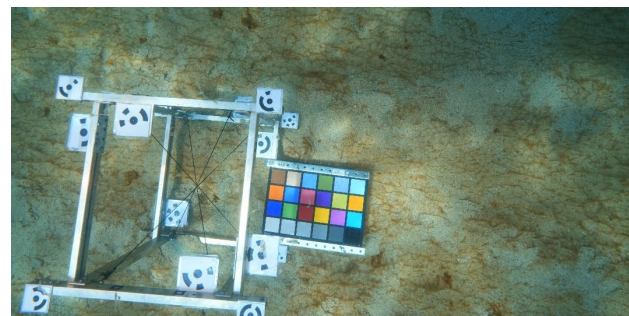
Figure 9. Original underwater image acquired with the ColorChecker positioned in the scene. This serves as the baseline for evaluating colour distortions before applying any correction.
