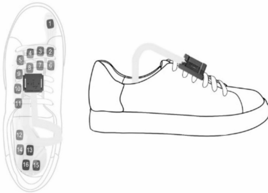
Fig. 2 Schematization of the experimental set-up: a 16-channel Pressure Insole (PI) is positioned inside each subject's shoe
