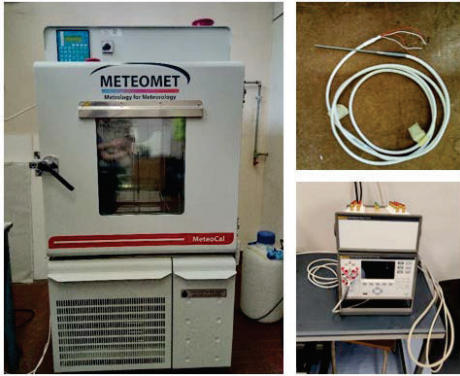
Fig. 2. INRiM laboratory setup: on the right the Kambic climatic chamber, whereas on the left the reference Pt100 and the Fluke DAQ temperature scanner.
