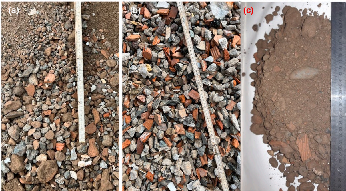
Fig. 5. Particle size distribution curves of the fill materials used in the experimental embankments, with detailed photographs of the aggregate mixtures: a) 0 ÷ 80 mm HM RA; b) 15 ÷ 30 mm JC RA; c) mix of excavated soils (50 %) and 15 ÷ 30 mm JC RA (50 %).
