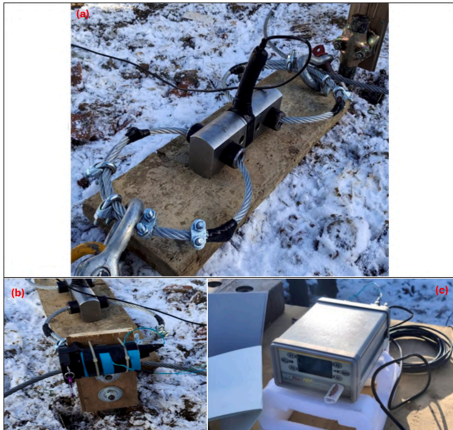
Fig. 9. Systems used to measure and record the variables of interest during pullout tests: a) 200 kN load cell; b) wire displacement transducer; c) data logger for data acquisition.
