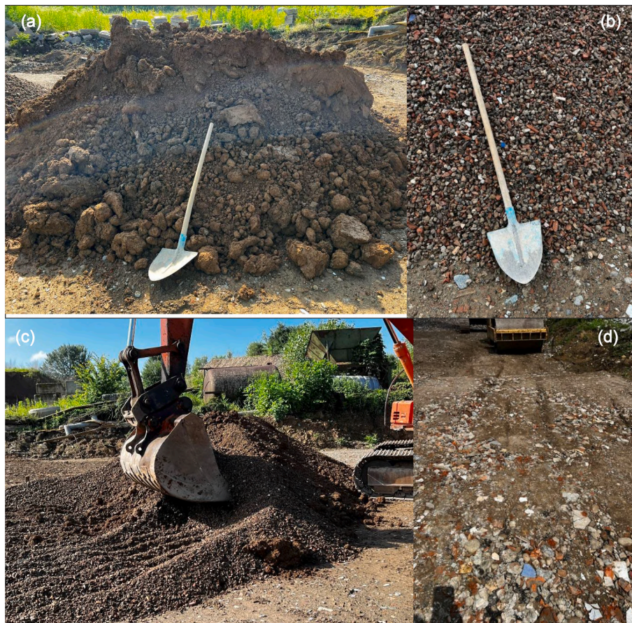
Fig. 1. Fill materials used for the experimental embankment. a) excavated soils; b) 15 ÷ 30 mm JC RA; c) mixture of excavated soil and 15 ÷ 30 mm JC RA; d) 0 ÷ 80 mm HM RA.
