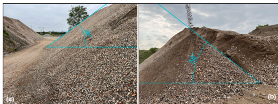
Fig. 6. Photographic representation of the granular material stockpiles used to evaluate the natural repose angle: (a) 15 ÷ 30_JC with a repose angle of 36°, (b) 0 ÷ 80_HM with a repose angle of 38°.
