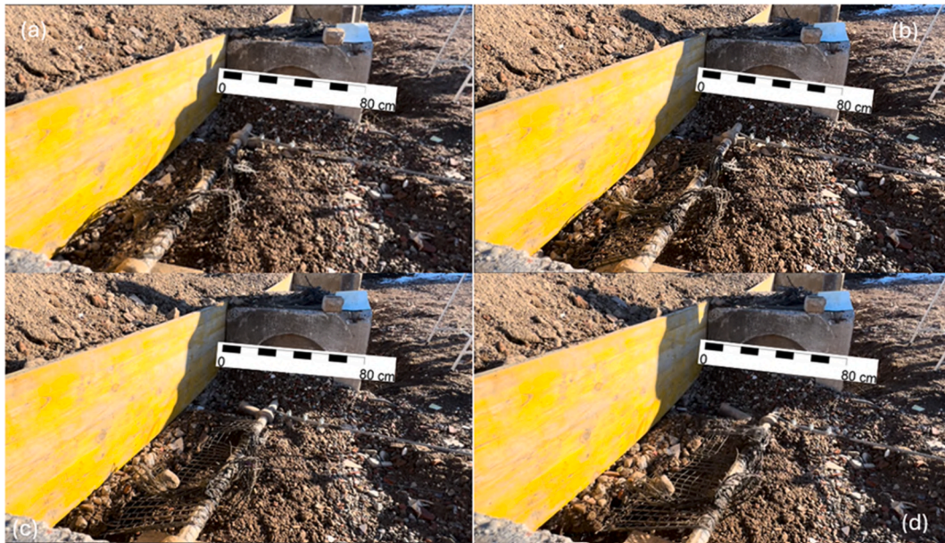
Fig. 11. Sequential frames captured at successive time intervals during the pull-out test C1. The graduated scale highlights the magnitude of the progressive displacement, providing a detailed visualisation of the phenomenon’s evolution. Notably, the progressive pull-out of the geogrid is accompanied by the ejection of some RA clasts. A short video of the pull-out test is provided in the supplementary materials.
