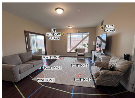
Fig. 2: Room layout indicating radars positions and activity locations.
