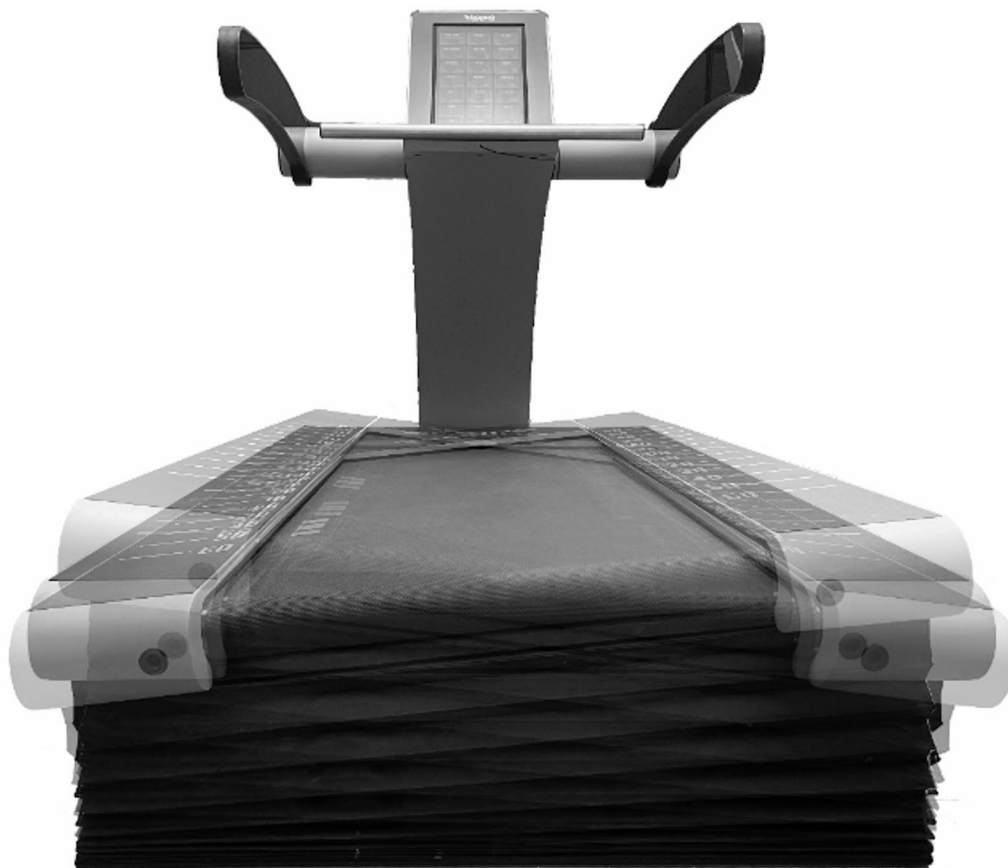
Fig. 2. Sketch of the treadmill used with the medio-lateral oscillations of +7/-7^\circ highlighted. Figure created from original photographs and processed using Adobe Photoshop (version 21.1.1) for illustrative purposes.
