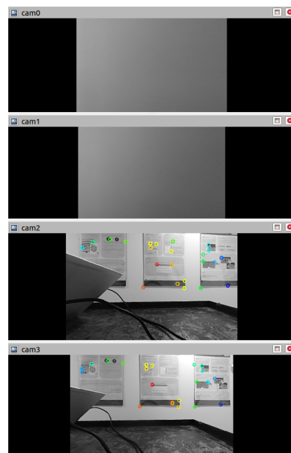
Figure 7. Multi-camera setup during robustness testing: cam0 and cam1 (Stereo 1); cam2 and cam3 (Stereo 2).
