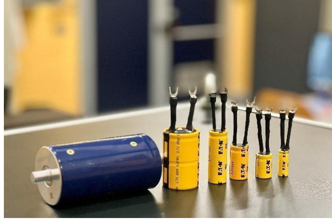
Figure 3.3. Samples of the SCs under test at INRIM. The fork terminals carry the current and are soldered to the SC terminals from which the sense terminals are derived by soldering, according to the 4-terminal method (see Sect. .3).
