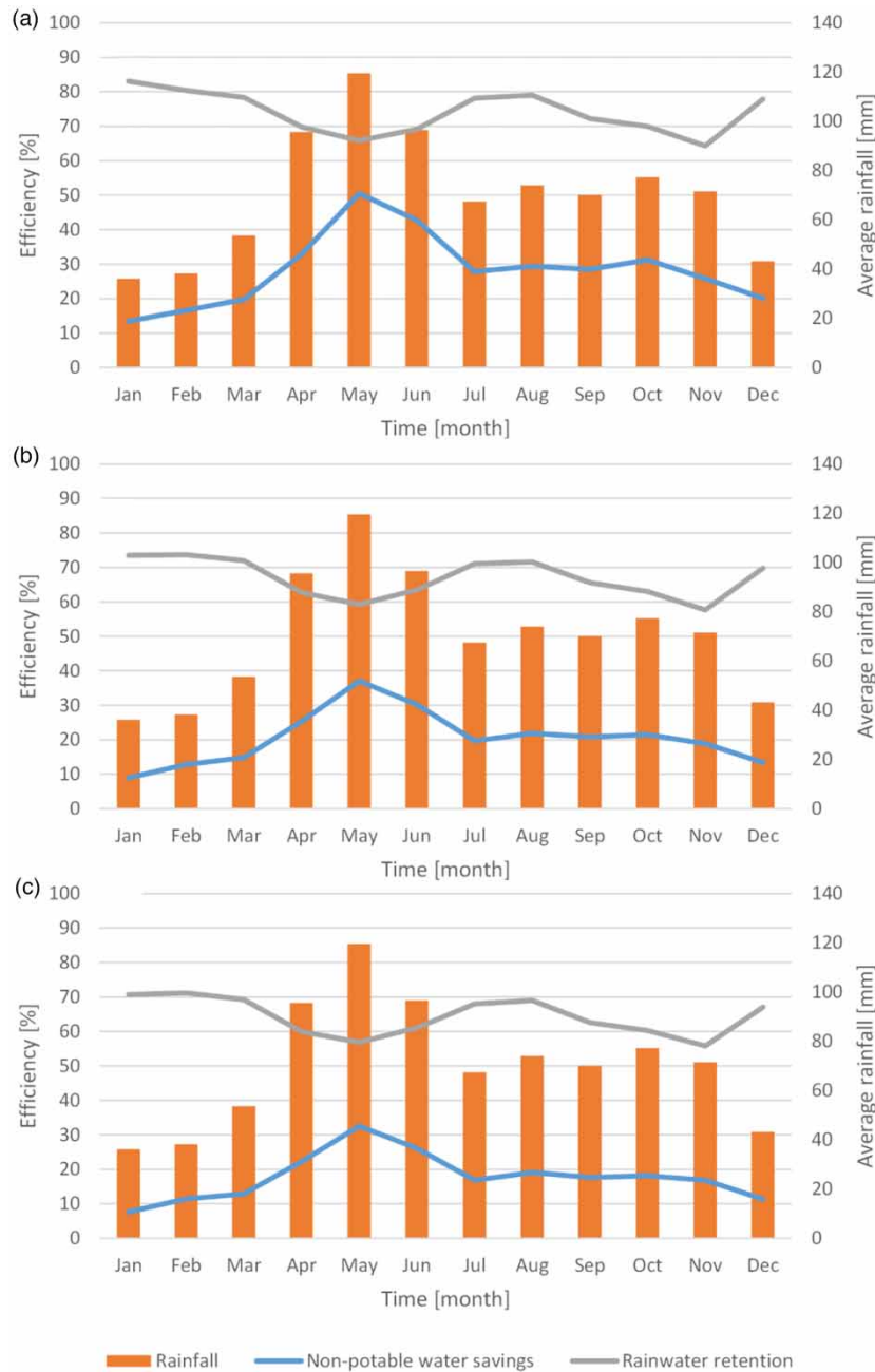
Figure 11 | Monthly variability of the efficiency of the RWH system associated with a green roof for building types 1 (a), 2 (b) and 3 (c) (tank capacity = 5 m 3 ).
