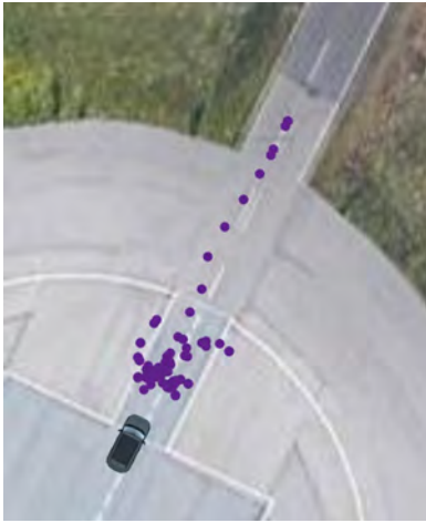
Fig. 3: Replay of a CAN trace with a perception of a pedestrian sensed by the equipped vehicle.
