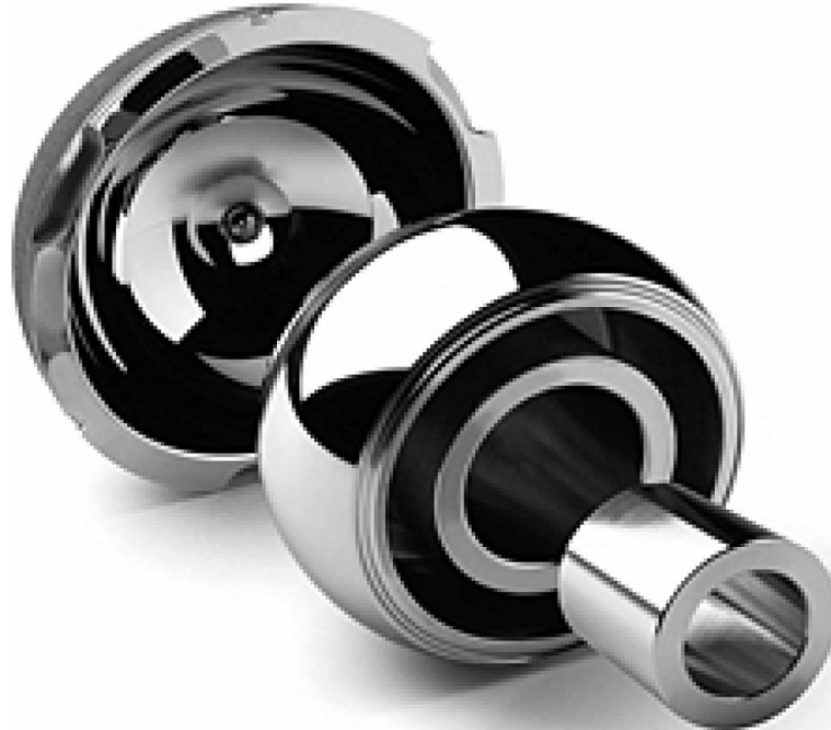
Figure 1. 5 Femoral bearing head and cups made from the F799 CoCrMo alloy. Image taken from [1]
