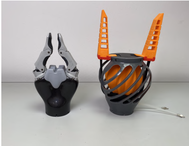
Figure 2.18: The BiSoft.Q Gripper compared to the Kinova KG2.
