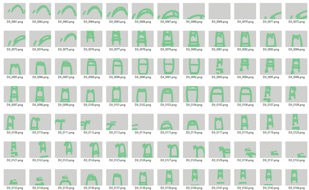
Figure 8. Preview of the automatically generated .png labels for the synthetic images dataset.
