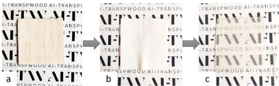
Figure 4: Main steps: balsa wood (a), delignified balsa wood (b), and transparent balsa wood. Reproduced from Kivikytö-Reponen et al., 2024 under CC-BY licence.
