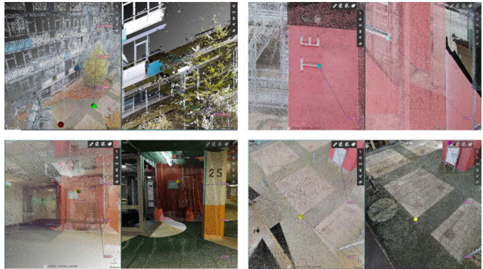
Figure 10. Example of common points chosen as a reference for the N-point alignment.
