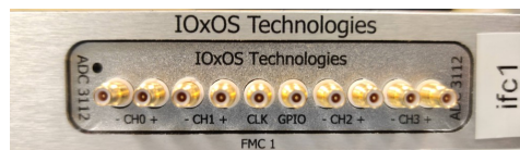
Fig. 2.9 ADC_3112 front panel with the SSMC connectors.
