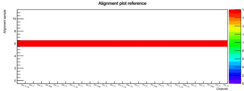
Fig. 3.26 ZDC ideal alignment plot using the reference signal for calibration.
