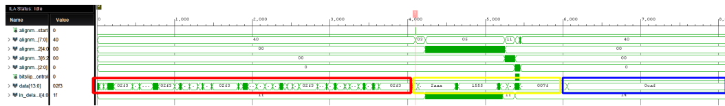
Fig. 4.15 Calibration example performed with hardware starting from a not calibrated configuration. The interesting areas, before, during, and after calibration are highlighted respectively in red, yellow and blue.
