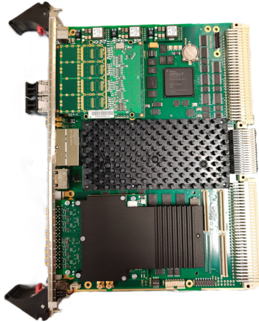
Fig. 2.10 IFC_1211 from IOxOS with two FPGA Mezzanine Card (FMC) modules. The one at the top hosts 4 Small Form-factor Pluggable+ (SFP+) connectors of which only two are populated. The one at the bottom is an ADC_3112 from IOxOS.
