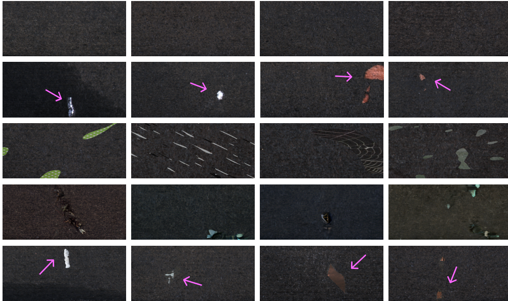
Figure 3.7 First row displays some negative samples from the KSDD2 dataset. Instead, the second row shows some images of positive samples from the same dataset. In the third row, we show the MemSeg-generated defect samples. The fourth row shows In&Out generated defect samples. Lastly, the final row showcases images generated with DIAG . Notably, the defect images that DIAG generated are more realistic and in-distribution.
