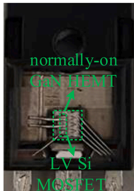
Fig. 4. Photo of a decapsulated cascode GaN device.
