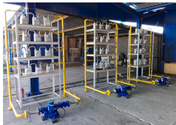
Fig. 2. The SGWT test bench to perform the ageing test of distribution gas meters.
