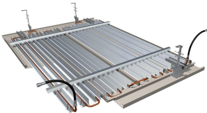
Figure 17: Example of a cooling panel.
