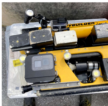
Figure 6. Cameras and lights, mounted on the side of the ROV.
