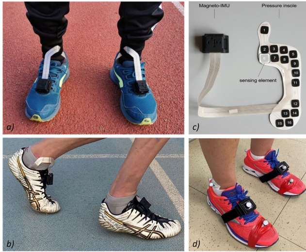
FIGURE 5. Experimental setup used in slow running speed dataset (Fig. 5a,c), moderate running speed dataset (Fig. 5d) and fast running speed dataset (Fig. 5b,c). All the setups included two shoe-mounted inertial sensors. In slow and fast running speed datasets a pressure insole was inserted in each shoe and used as a portable gold standard for running temporal parameters. In the moderate running speed dataset (Fig. 5d), trajectories of the retro-reflective markers of the stereo-photogrammetric system were used as a gold standard for the identification of running temporal parameters.
