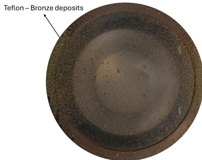
Figure A.2. Teflon – bronze deposits on the piston quartz window.
