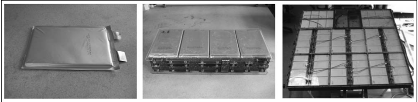
Figure 1. The three main assembly levels of the battery pack (cell, module, pack) of an electric bus [36].
