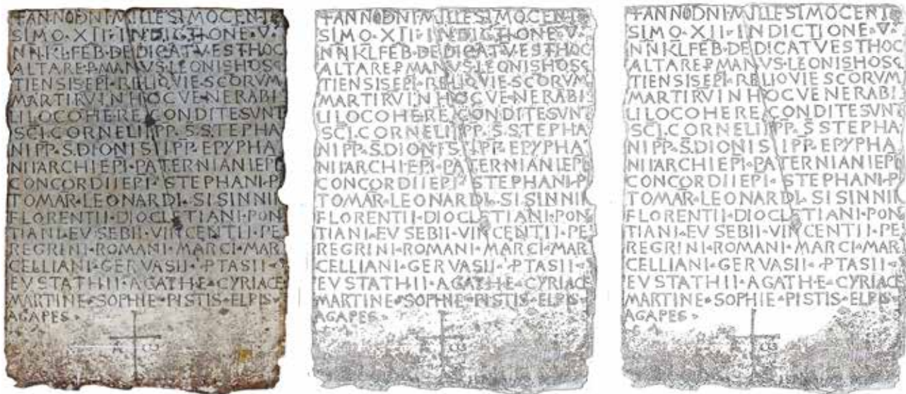
Figure 13. Image processing steps: contrasted image, features extracted and outliers cleaned.
