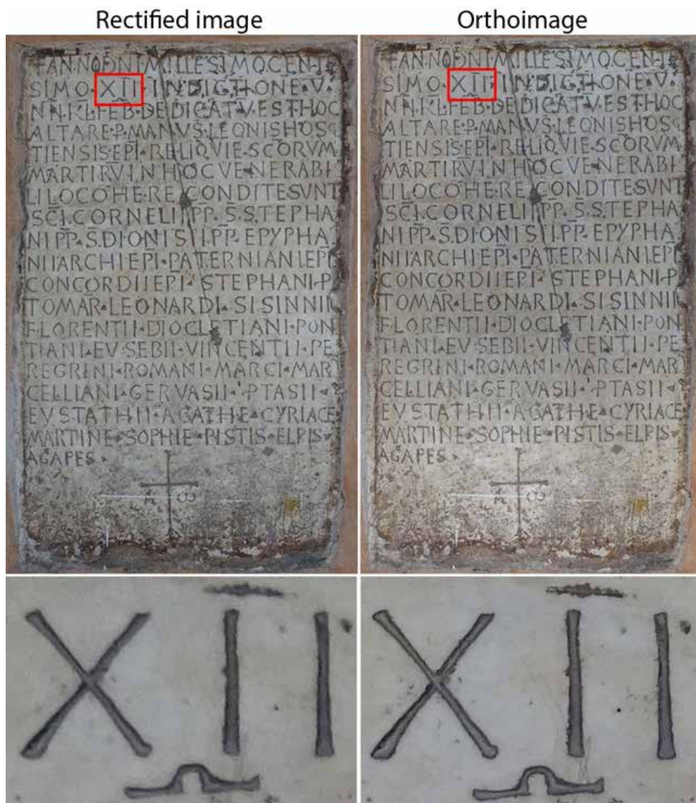
Figure 6. Comparison between rectified image and orthophoto with relative details.
