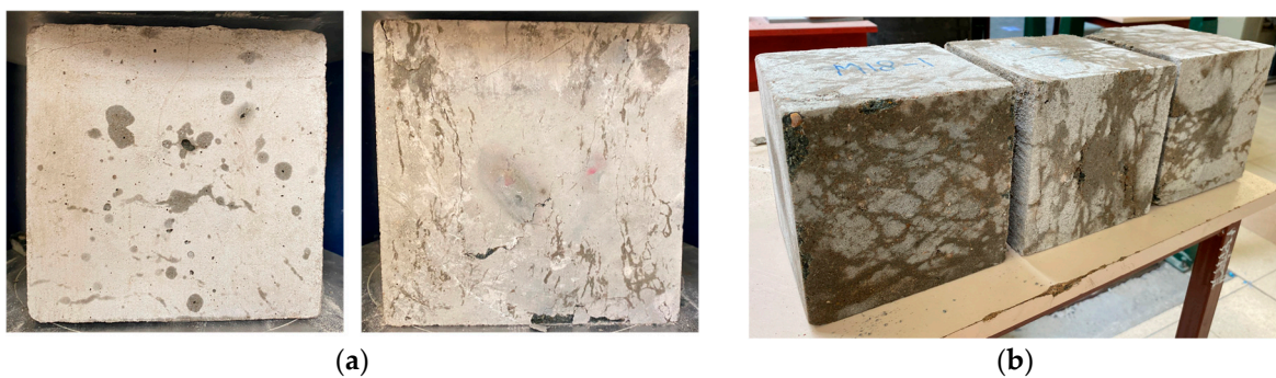
Figure 8. (a) Wet spots as an indication of capsule breakage during compression tests, (b) the spread of WRA via microcracks and capillary action.
