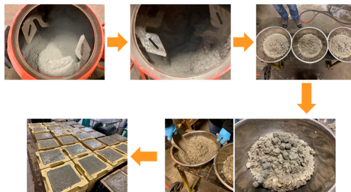
Figure 4. Procedure of casting the capsule-based concrete.
