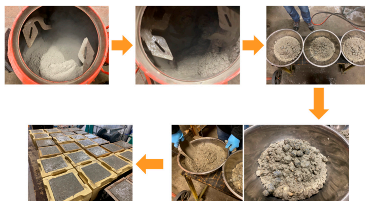
Figure 4. Procedure of casting the capsule-based concrete.
