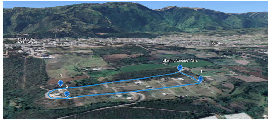
Figure 12. Route in Ibarra, Ecuador, used to compare vehicles fitted with original and modified suspensions under the same test conditions. Satellite image downloaded using Google Earth. Straight section followed by a sharp turn in (1), wide turn between points (2) and (3).
