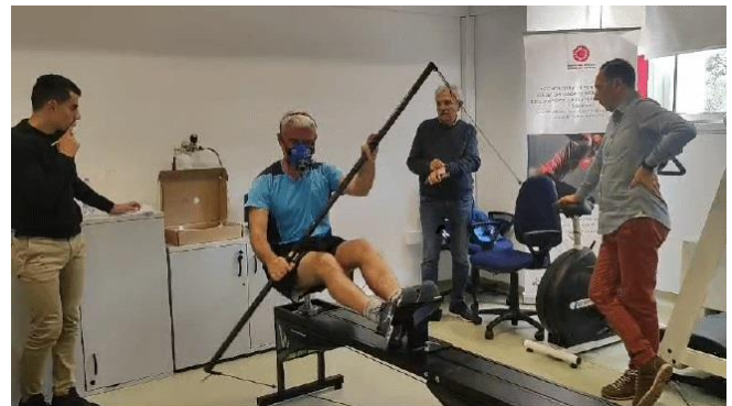
Figure 1 The athlete while paddling on the kayak lab simulator is shown. The bar he holds simulates the paddle in the act of pushing it down and back with his right hand. It is attached to the manually variable mechanical resistance system located in the anterior side of the ergometer by two ropes at the ends. On his face, the athlete wears a mask connected, by thin tubes, to the gas analyser for collecting respiratory and metabolic variables as: oxygen consumption, carbon dioxide production and pulmonary ventilation.
