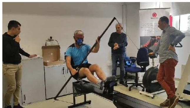
Figure 1 The athlete while paddling on the kayak lab simulator is shown. The bar he holds simulates the paddle in the act of pushing it down and back with his right hand. It is attached to the manually variable mechanical resistance system located in the anterior side of the ergometer by two ropes at the ends. On his face, the athlete wears a mask connected, by thin tubes, to the gas analyser for collecting respiratory and metabolic variables as: oxygen consumption, carbon dioxide production and pulmonary ventilation.
