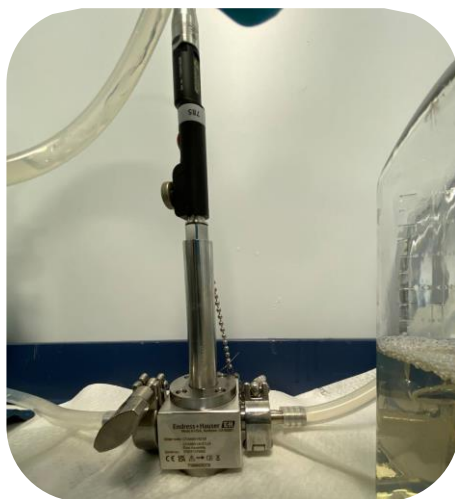
Figure 16: Raman flow cell used for in-line measurements installed in the GPD department of Guidonia Montecelio Merck site
