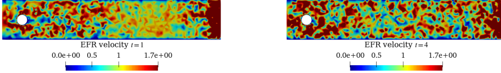
FIGURE 13. Experiment 1. Velocity profiles for EFR simulation on the coarse mesh (M1) for t = 1 and t = 4 , left and right plots, respectively.
