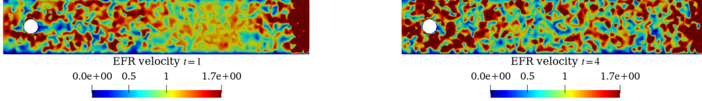
FIGURE 13. Experiment 1. Velocity profiles for EFR simulation on the coarse mesh (M1) for t = 1 and t = 4 , left and right plots, respectively.
