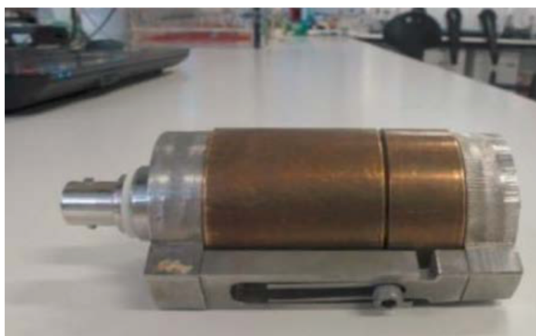
Figure 3 - 6. Barrel cell used for conductivity measurements.
