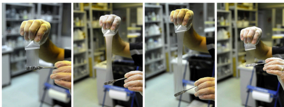
Figure 2 - 1. UV-crosslinked PEO–LiTFSI–C4mpyrTFSI ternary SPE subjected to manual elongation. Adapted from Ref. 11, with permission from Journal of Power Sources. Copyright 2010.
