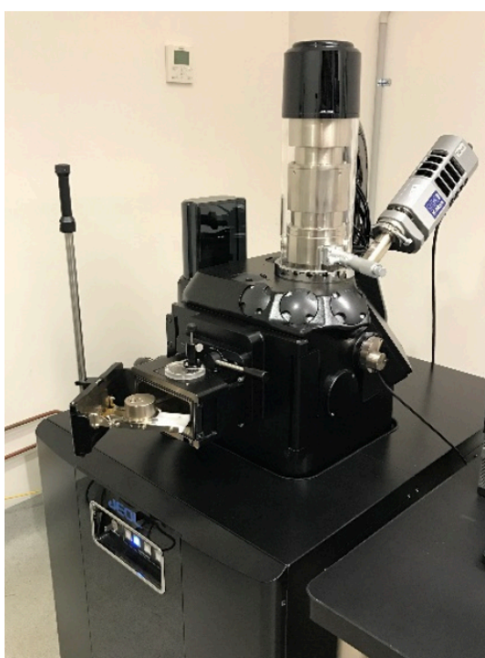
Figure 3 - 3. The JEOL JSM-IT300 SEM used in this PhD thesis.
