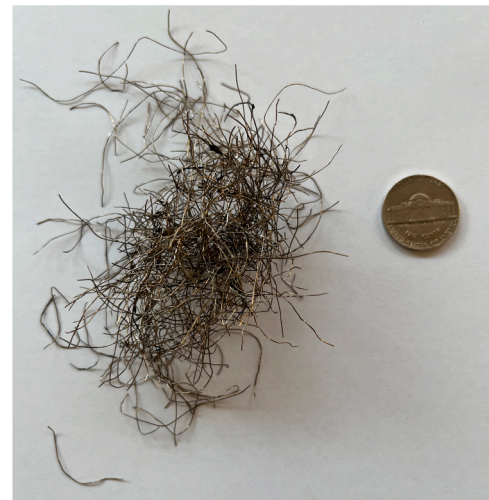
Fig. 2. Recycled steel fibers (RSF) from end-of-life tires.
