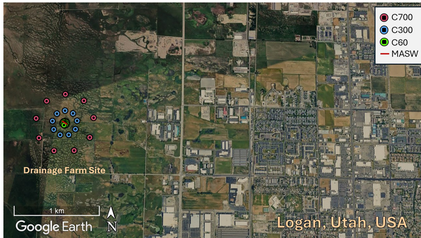
Figure 10. Plan view of the MASW and MAM arrays employed for testing at the Drainage Farm Site in Logan, Utah, USA. The concentric MAM arrays featured diameters of 60 (C60), 300 (C300), and 700 m (C700), while the MASW array comprised 24, 4.5 Hz vertical geophones, spanning 46 m.
