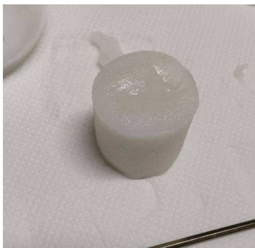
Figure 9. Slurry extracted from the extruder after a printing test.
