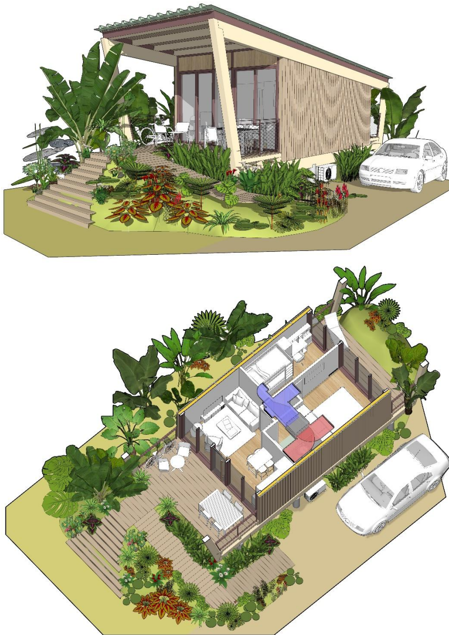
Fig. 3. 3D axonometric views of the minimal residential unit
