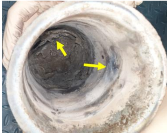
Figure 69. Bluish patina and oxide skins into the Alumina crucible after atomization of ingot AlSi9Cu3(Fe).
