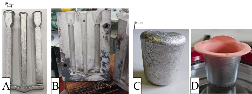
Figure 22. Casted samples and mould. A: samples for mechanical tests; B: mould for casting samples for mechanical tests; C: sample for microstructural analyses; D: crucible used for casting samples for microstructural analyses.
