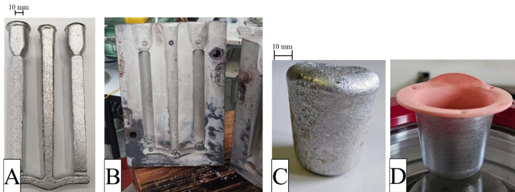
Figure 10. Cast and mould. A: cast for mechanical samples; B: mould to cast mechanical samples; C: cast for microstructure characterizations; D: crucible used to cast samples for microstructural characterizations.
