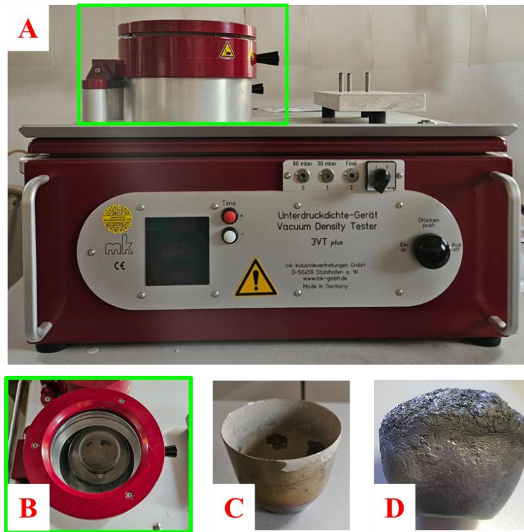
Figure 9. Dross and Straube Pfeiffer tests apparatus. A: Instrument; B: chamber to perform tests; C: crucible for Dross test and Straube Pfeiffer test; D: obtained sample.
